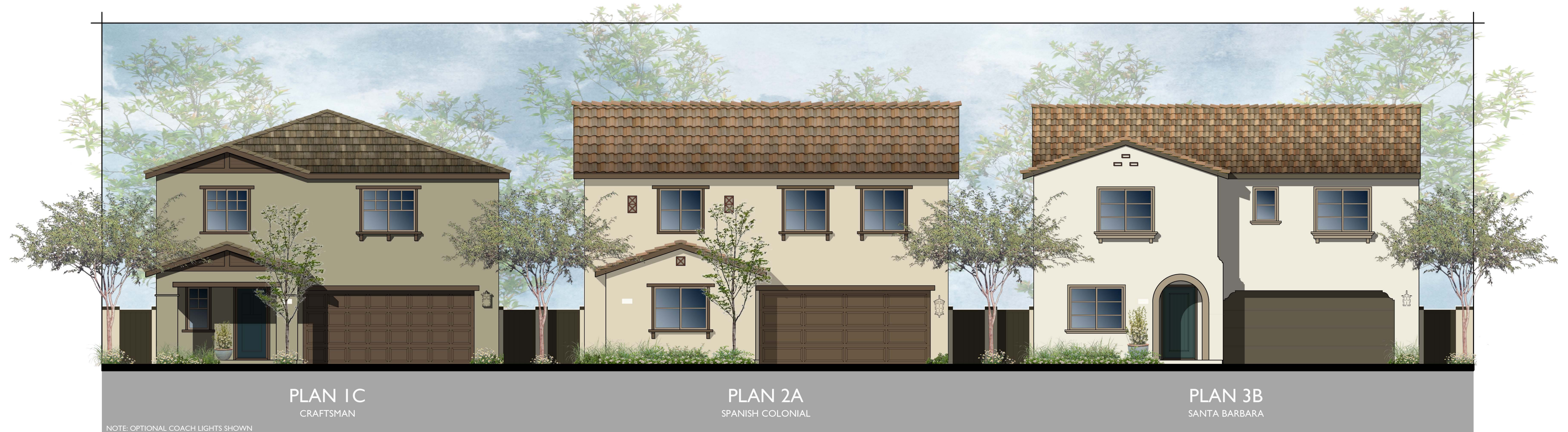
ROOF PLAN C PITCH: 4:12 RAKE: 12" EAVE: 12" ROOF MATERIAL: CONCRETE FLAT TILE
