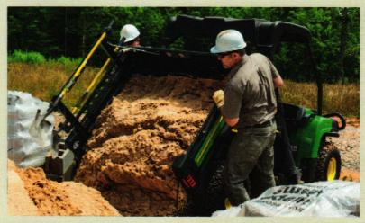
Generous Cargo Box is built with tough, composite materials. Its 16.4 cu. ft (.56 cu. m.) can handle 1,000 lb. [450 kg] easy.
